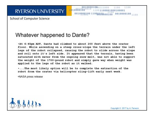
The most likely cause for the collapse was a problem with the software used to achieve the autonomous walking behaviour. The algorithm assumed that the foot of the leg being moved would be place in snow. In order to break the crust of the snow the leg was pushed hard and down. This apparently had been simulated unfortunately the sides of the volcano were rather muddy...who would have figured that a volcano would melt the snow?
