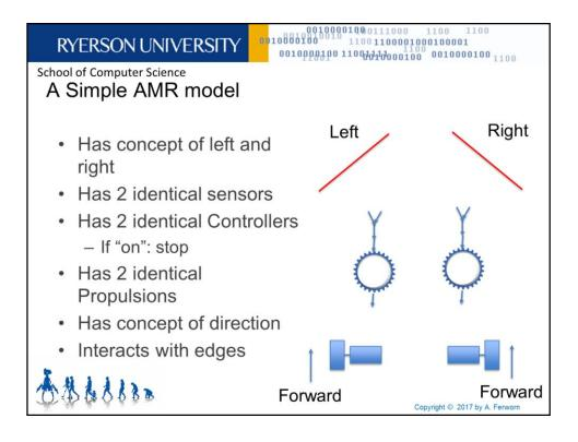
If we have a left and a right side of our problem we can start to reason about our robot that also has a left and right side. Really the only thing that has not been defined is how the controllers are connected to the propulsion. Let us assume that the left controller is attached to the left propulsion (assume the same for the right side) and we will also assume that the direction of motion for the respective propulsions is forward.
