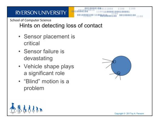
•Sensor placement is critical: Any vehicle motion must be covered by sensor feedback. For example, if the vehicle detects an edge and moves backward and there is another undetected edge to its rear, the result will be catastrophic system failure.
