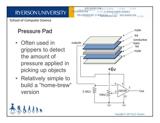
LM339 is a quad comparator circuit. Output will be +6V
