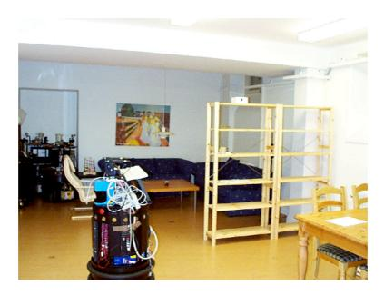
Fig. 1. The living room. Our main lab has been turned into a living room in which there are sofas, tables, book-shelves, and so on, to make it possible to test the robot in a realistic setting.
